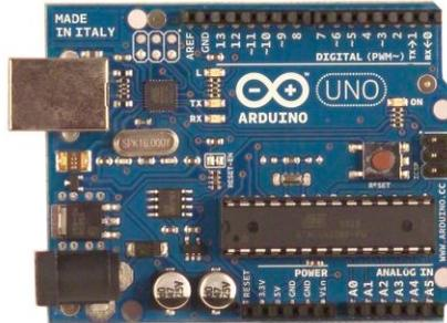
**FIG.2.1: Arduino microcontroller**
